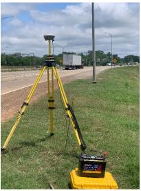
In order to establish the baseline, we will set an autonomous base point near the bridge. Then using RTK, we will tie surface features along the bridge and any monuments found along the baseline. Once the baseline is established relative to the base point, RTK can be used to determine the exact location of the predetermined offsets along the cross-sections.
