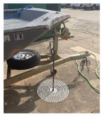
determined, a bar check will be taken to verify the calibration.
